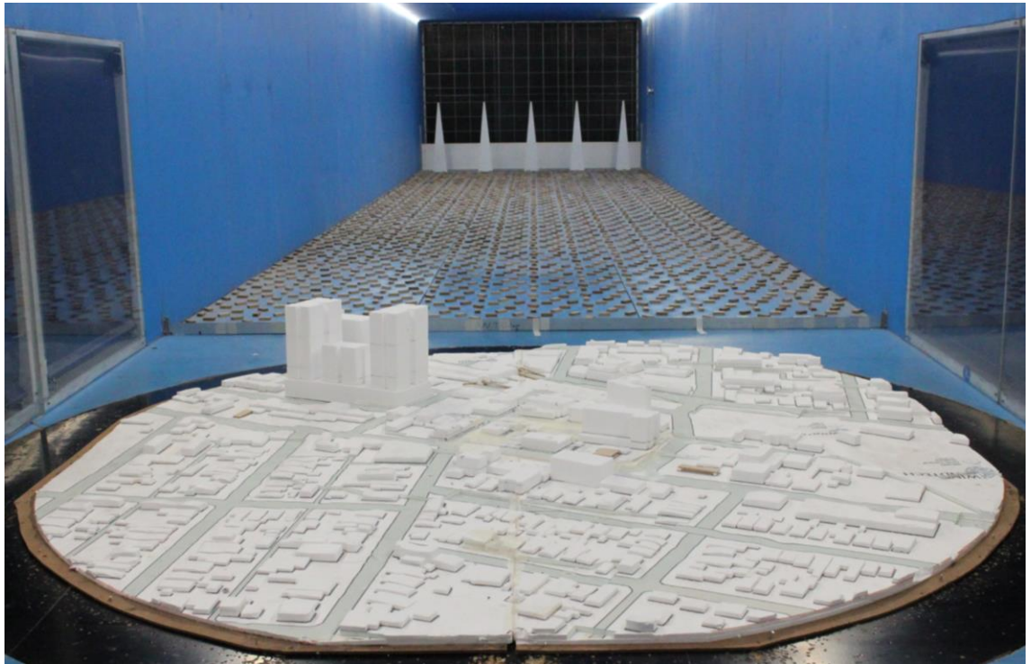
Figure 1g: Photograph of the Wind Tunnel Model (existing scenario, view from the north-west)
