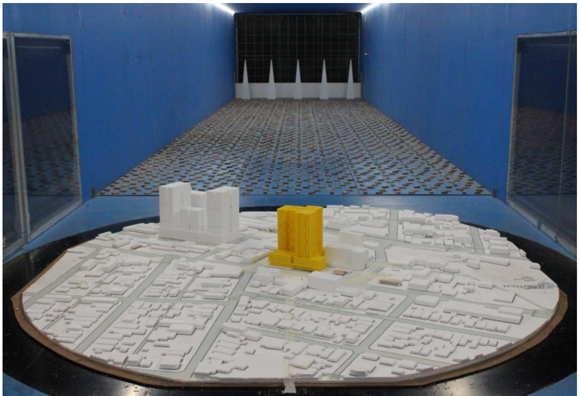
Figure 1c: Photograph of the Wind Tunnel Model (proposed scenario, view from the north)
