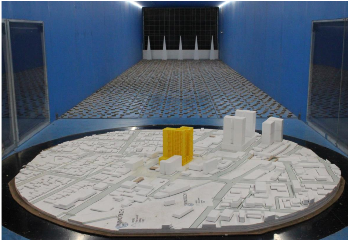
Figure 1d: Photograph of the Wind Tunnel Model (proposed scenario, view from the west)
